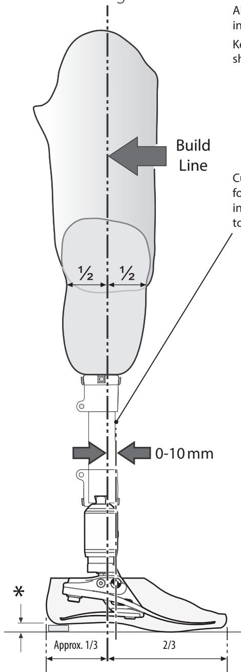
Align transfemoral devices according to fitting instructions supplied with the knee.
