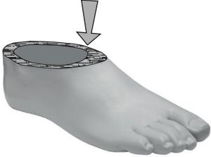
The diagram shows a foot wearing a white cosmetic bootie. A grey arrow points to the top surface of the bootie, indicating the area to be sanded.
